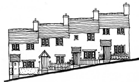
A strip elevation indicating small houses stepped against the contours. Avoid attempting to make a sloping site flat - work with the character of the site - not against it!
