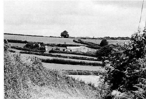
Siting large structures below the skyline helps to reduce their impact.
